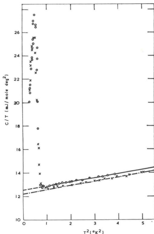
Fig. 6. Heat-capacity data for the 5- and 7-at.% Mo alloys in zero field showing the superconducting transition: O 5 at.%, X 7 at.%.
