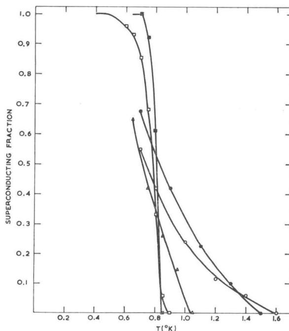
Fig. 7. The superconducting fraction as a function of temperature as determined from the heat-capacity data. Mo content in at.%, O 0.3, ● 0.6, △ 3, □ 5, ■ 7.
