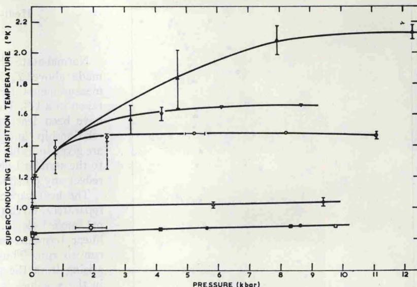
FIG. 3. Magnetically determined transition temperature as a function of pressure: Mo content in at.%,  $\Delta$ 0.3,  $\nabla$ 0.6,  $\square$ 3,  $\bullet$ 5,  $\blacksquare$ 7.
