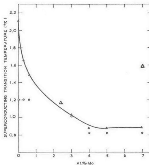
Fig. 2. Magnetically determined transition temperature at  $P=0$  and 10 kbar as a function of Mo content:  $\circ$  ( $P=0$ ),  $\triangle$  ( $P=10$ ) kbar.  $\triangle$  data of Chandrasekhar and Hulm (Ref. 13).
